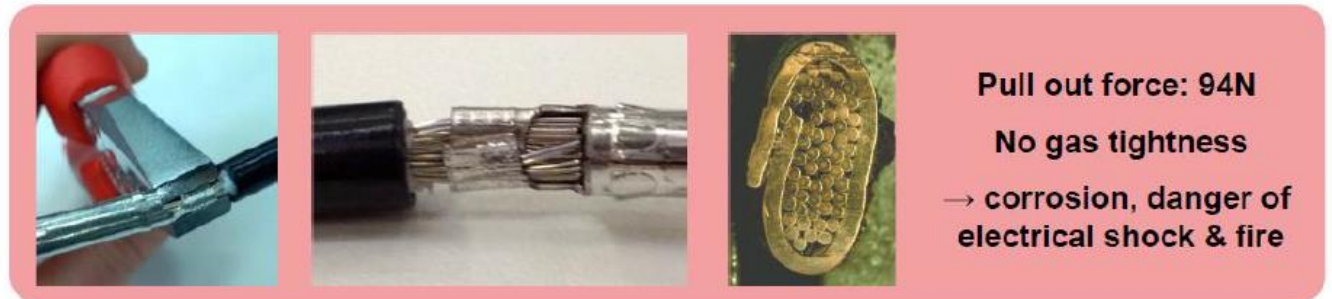
Figure 5: Comparison between connection with correct and incorrect crimping pliers (Berginski, 2013)
